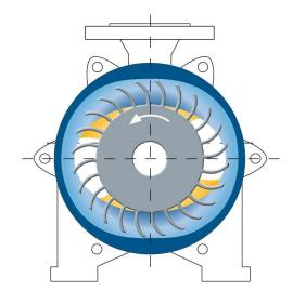
For realization of high compression pressures at large volumetric flow rates the liquid ring compressors are developed with a combination of single and double acting design. The machines are working almost with an isothermal three-stage compression.
